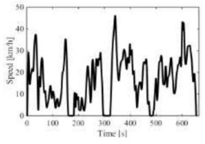
Fig. 4. Overall driving cycle of xi'an
